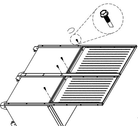
Insert the Hexagon bolt with flange screw(M6X25) through the back of hauger boards, and into the side of wooden work plate. Tighten securely.
