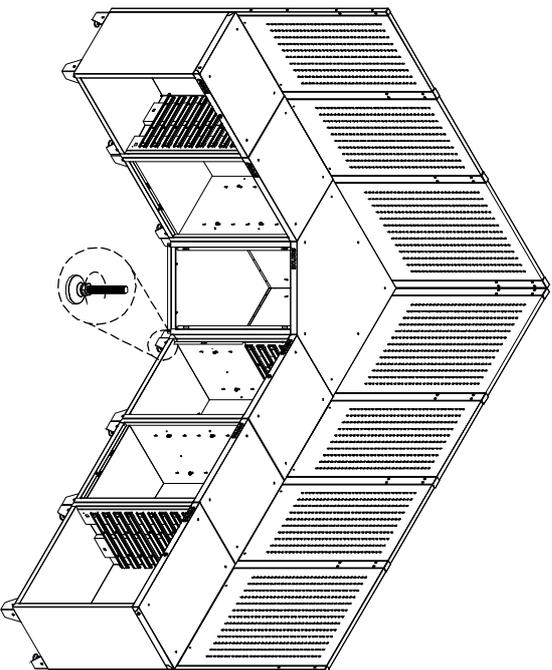
B) To connect each cabinet by hex flange bolt ( M6x16 ) and hex flange nut. Tighten the screws securely.
