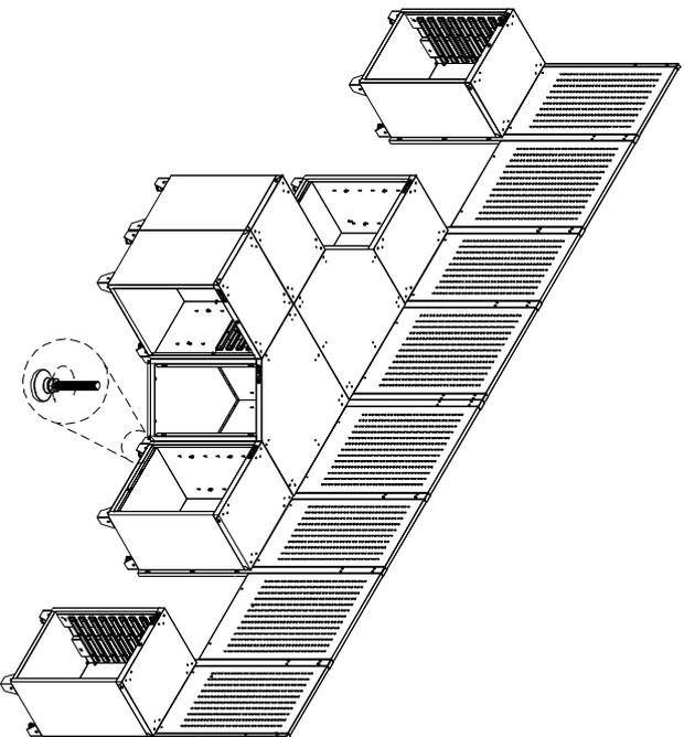
B) To connect each cabinet by hex flange bolt ( M6x16 ) and hex flange nut. Tighten the screws securely.
