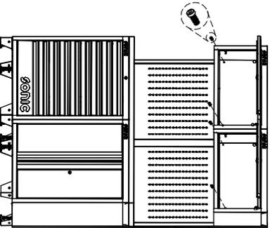
Insert the hexagon bolt with flange screw (M6X25) through the back of hauger boards, and into the side of SS work plate. Tighten securely.
