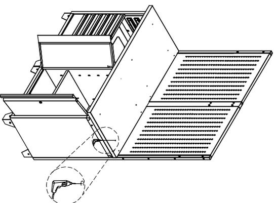
**5. PRE-DRILL HOLES OF SS WORK PLATE**
