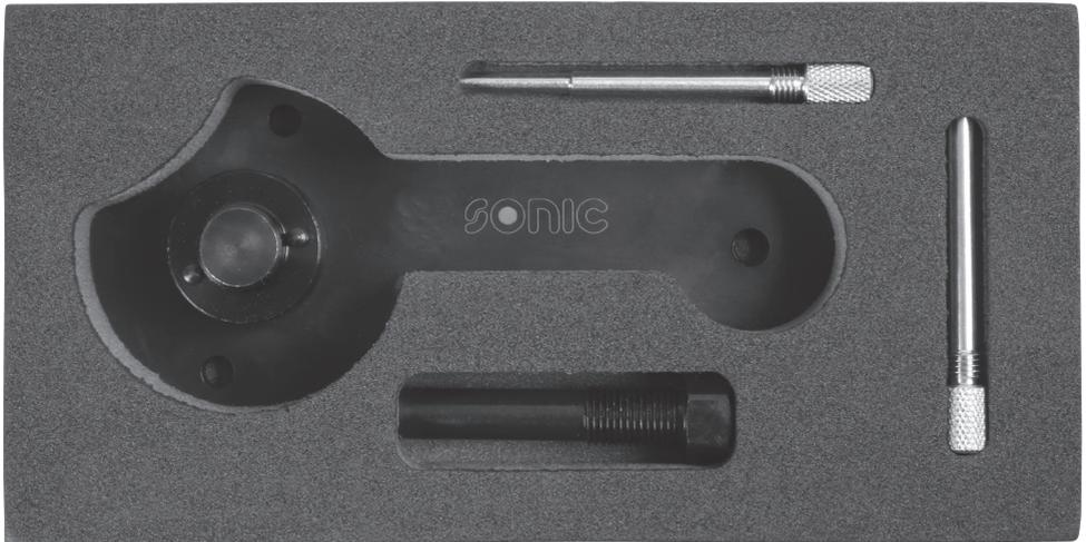
The 829125 timing tool kit provides the essential camshaft and crankshaft setting tools to allow replacement of the camshaft drive belt on the new (2012 onwards) VAG 1.4 TFSi petrol engines.
