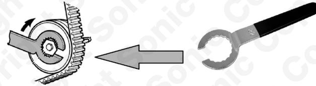
Component 5 - Front Pulley Holding Tool
