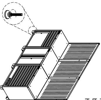
**5. PRE-DRILL HOLES OF SS WORK PLATE**
