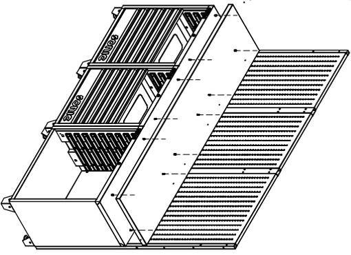
Insert the Hexagon bolt with flange screws (M6X25) through the back of hauger boards, and into the side of SS work plate. Tighten securely.
