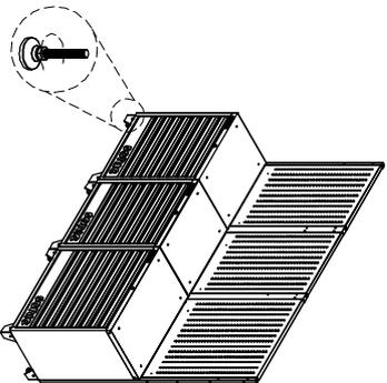
**4. PRE-DRILL HOLES OF SS WORK PLATE**
